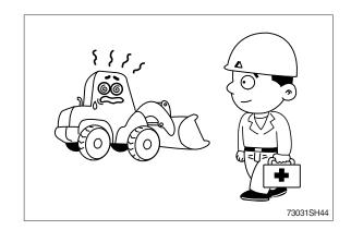
Park on a flat place for inspecting and repairing and properly TAG machine is not operational. (remove start key)
